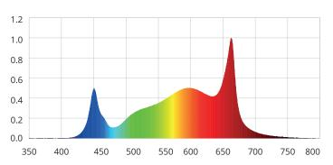
Our combination of white and red LEDs result in a relatively high ratio of blue light. Blue light keeps your crop compact in the vegetative stage and adds to an optimal morphogenesis and light interception by the plant.
